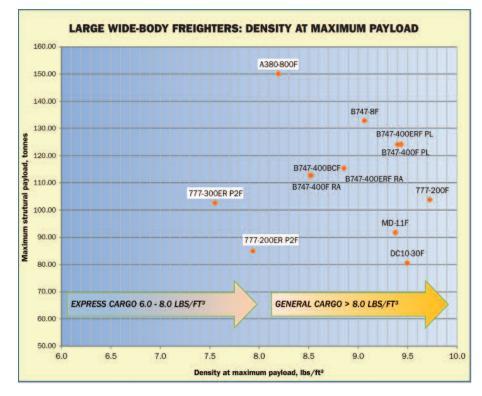
greater volumetric payloads than the -200ER P2F aircraft at all packing densities above 7.93lbs per cu ft. Significantly, the 777-300ER P2F offers higher volumetric payloads than the -200F at all densities up to 9.5 lbs cu ft, by virtue of its 26% volume advantage.
