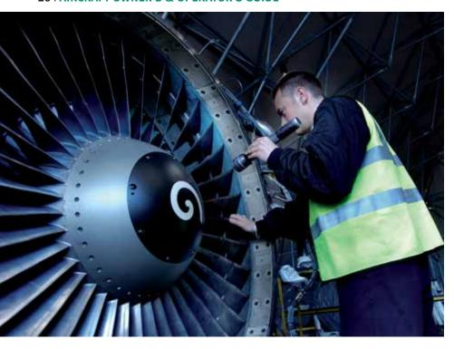
The CFM56-3 will have on-wing intervals of 5,000-18,000EFC if not limited by LLPs, depending on thrust rating and operating environment.
