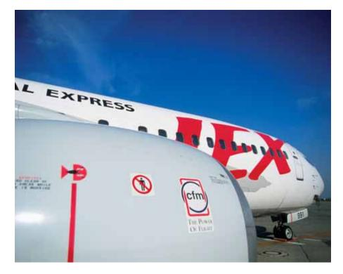
CFM56-3s rated at 22,000lbs & 23,500lbs thrust that operate in high temperatures have the most to gain from the performance upgrade modifications. These increase EGT margin and so improve on-wing life.
