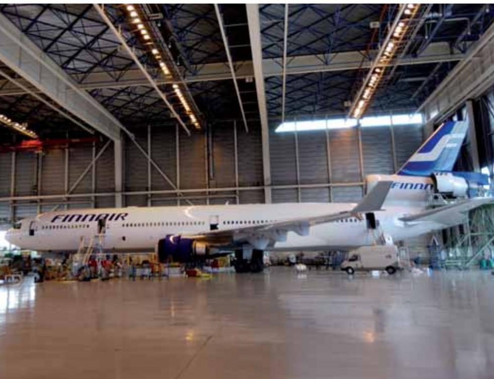
The MD-11's base maintenance programme is simple, with a series of four checks culminating in a heavy check. The C4 check is used to refurbish the aircraft interior and overall usually is a large workscope. The aircraft has so far demonstrated a low non-routine ratio.
