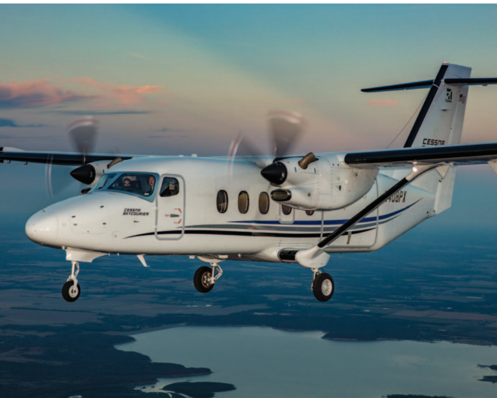
The Cessna Skycourier when configured as a freighter is capable of carrying three LD-3 or four LD-2 universal loading devices and has a gross payload of 6,300 lbs. Launch customer FedEx currently operates the single pilot certified type on its 190nm route between Orlando and Tallahassee.
