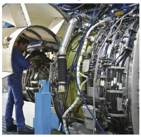
performance restoration will use about 3,000MH, while a core overhaul will use 3,600-4,000MH. At typical fully burdened labour rates of \$75-100 per MH, this is equal to \$225,000-400,000.
