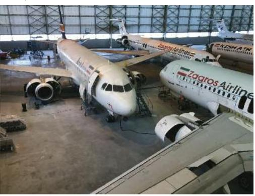
will incorporate the 1C and 2C tasks which have thresholds of 7,500FH and 15,000FH respectively; and the third C check will consist of 1C and 3C tasks in addition to 6YE structural items, thereby making it a more extensive check.
