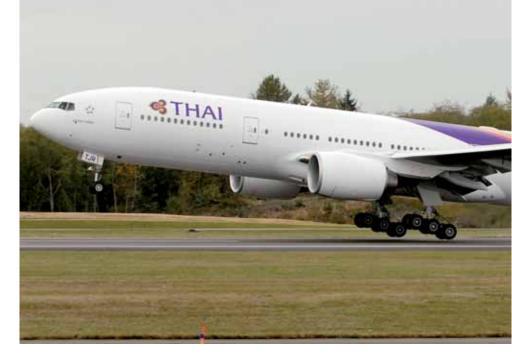
GE developed the GE90-115 for the 777-300ER and de-rated the engine design for the -200LR and 777F. Developments included aspects that improve fuel efficiency, thrust and the noise levels of the engines. The improved combustor means that the engine is producing no more than 50% of the carbon dioxide levels currently allowed by international standards.
