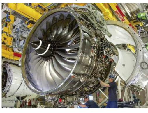
missions, but resulted in few cancellations. Routine tasks that have been added since service entry include IPT stage 2 blades inspection before 1,300EFC since new, and inspection of the LPT module within 1,500EFC.
