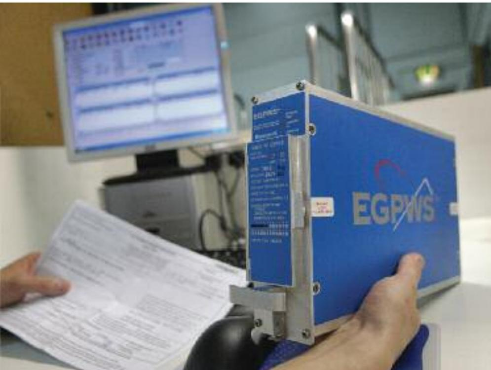
*Key aspects of rotatable management include the testing and repair of unserviceable components. Documentation management is also important. A serviceable part must have appropriate certification and trace paperwork.*
