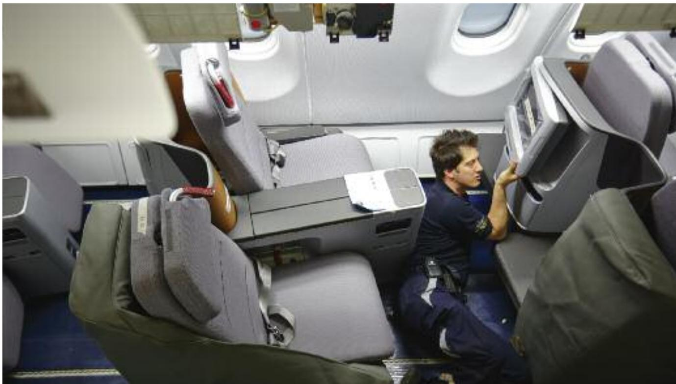
require inspection of seat structure, seatbelt integrity and attachment of the seat to the floor rails every 36 months.
