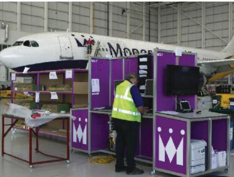
effectiveness that allows an operator's fleet to achieve shorter downtimes and more efficient maintenance. Paperless maintenance increases a mechanic's labour efficiency. A mechanic would not have to continually revert to a fixed, central computing station, for example, to input data or look up a manual reference as is typically the case. This lengthens the time spent on tasks.
