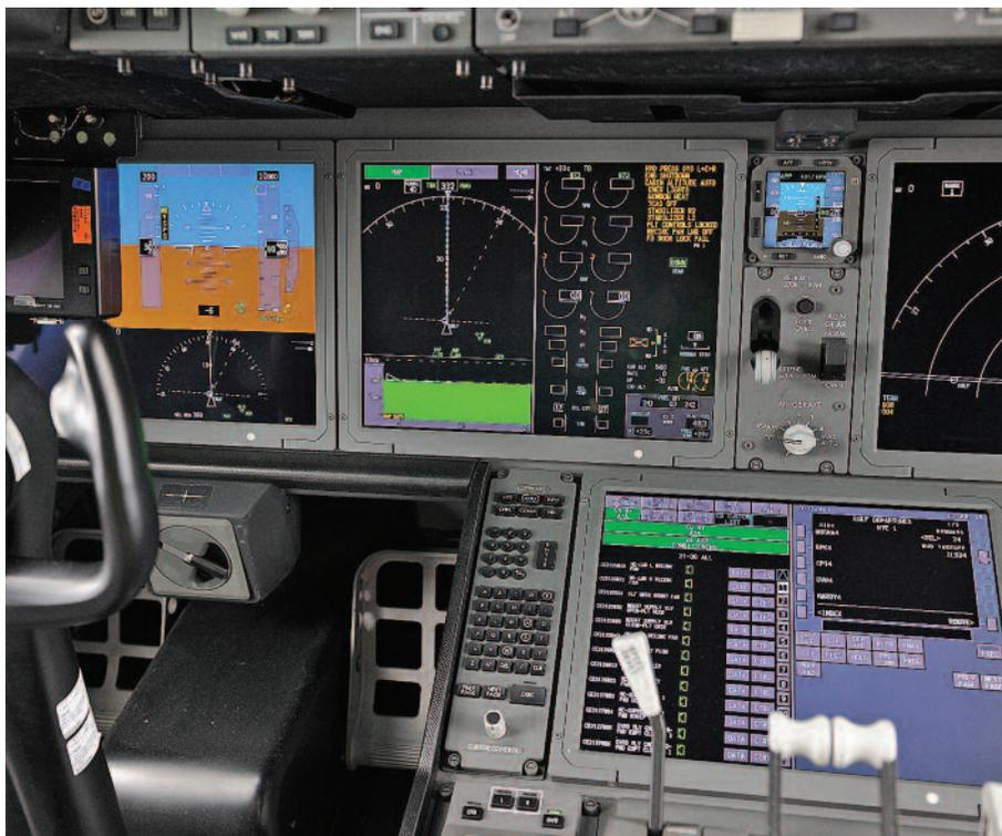
indication and crew alerting system (EICAS) screens on the flightdeck.
