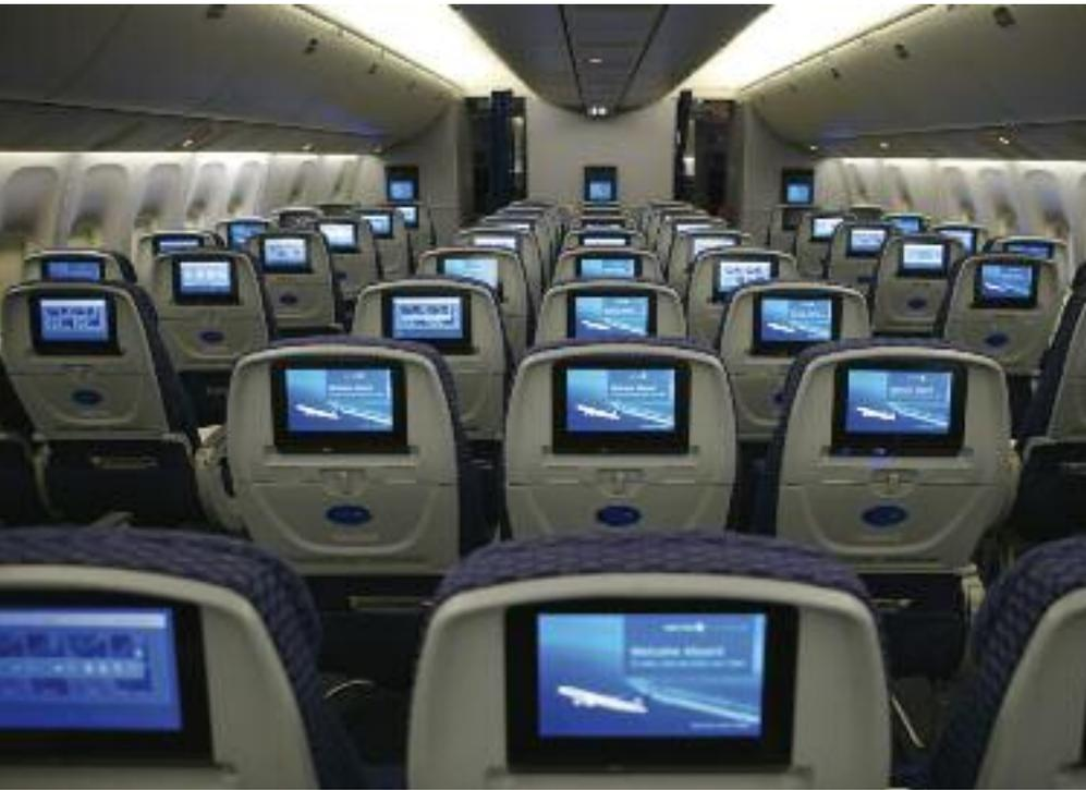
Westjet's new IFE system is Westjet Connect, provided by Panasonic. This is combined with in-cabin WiFi connectivity for use with PEDs, which is Panasonic's eXConnect system. It was launched in July 2015, and is being installed on all of WestJet's jet aircraft.
