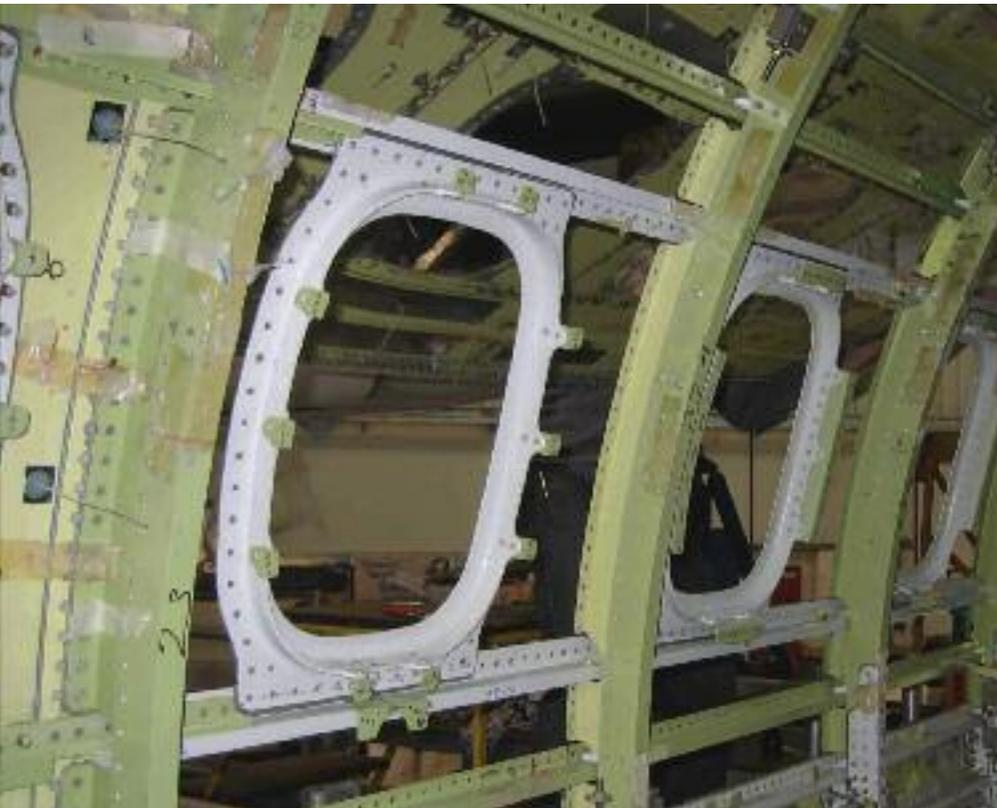
had to be carried out no later than the second base check or within 72 months, and concerned all ATRs, for example 42-500s up to MSN 641. Higher aircraft MSN were fitted with the MPC as standard on the production line. “Retrofitting the MPC took about 350MH,” says Peters.
