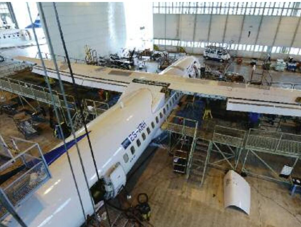
The third base check, or Base 3 check, which would be up to another two years later, and so at up to the sixth year of operation, would combine the 1C, 2C, 1YE, 2YE, and 4YE tasks. The 8YE tasks may also be brought forward at this check (see table, page 50). This would result in a package requiring a total of 1,300MH for inspections and access for these routine tasks.
