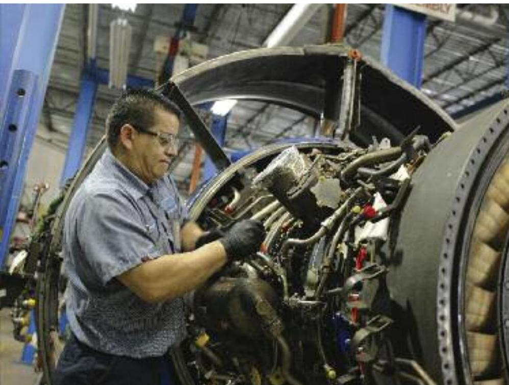
SR Technics offers the full range of services, including engine and module overhaul and repair, provisioning spare parts, and performing piece part repairs. Most of this work takes place in-house.
