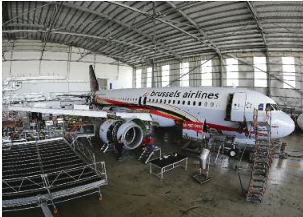
Once the A320 meets and exceeds 20,000FC, an increase in structural and deep access-focused tasks will be gradually introduced.
