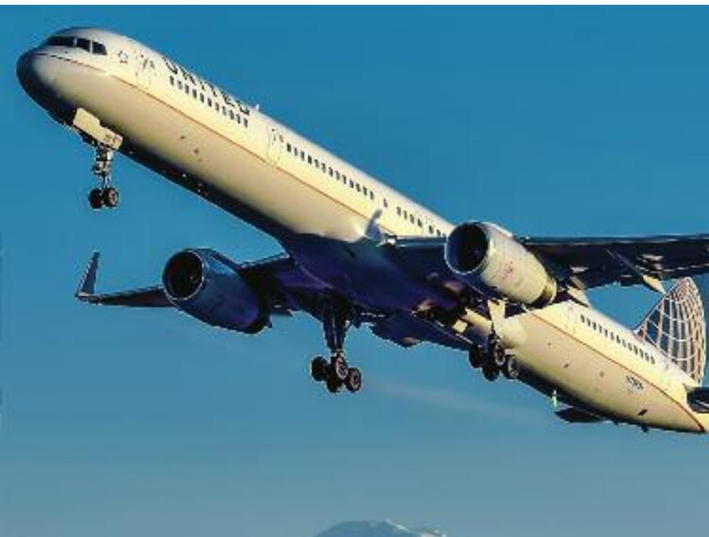
temperatures. At lower air densities the efficiency of aircraft engines is reduced. At an airport with a high elevation and/or higher ambient temperatures, an aircraft will need a longer take-off run than it would from an airport at sea level with standard temperatures. In some cases the take-off distance required to operate at MTOW from hot and high airports might not be available, and a payload and/or range restriction will apply.
