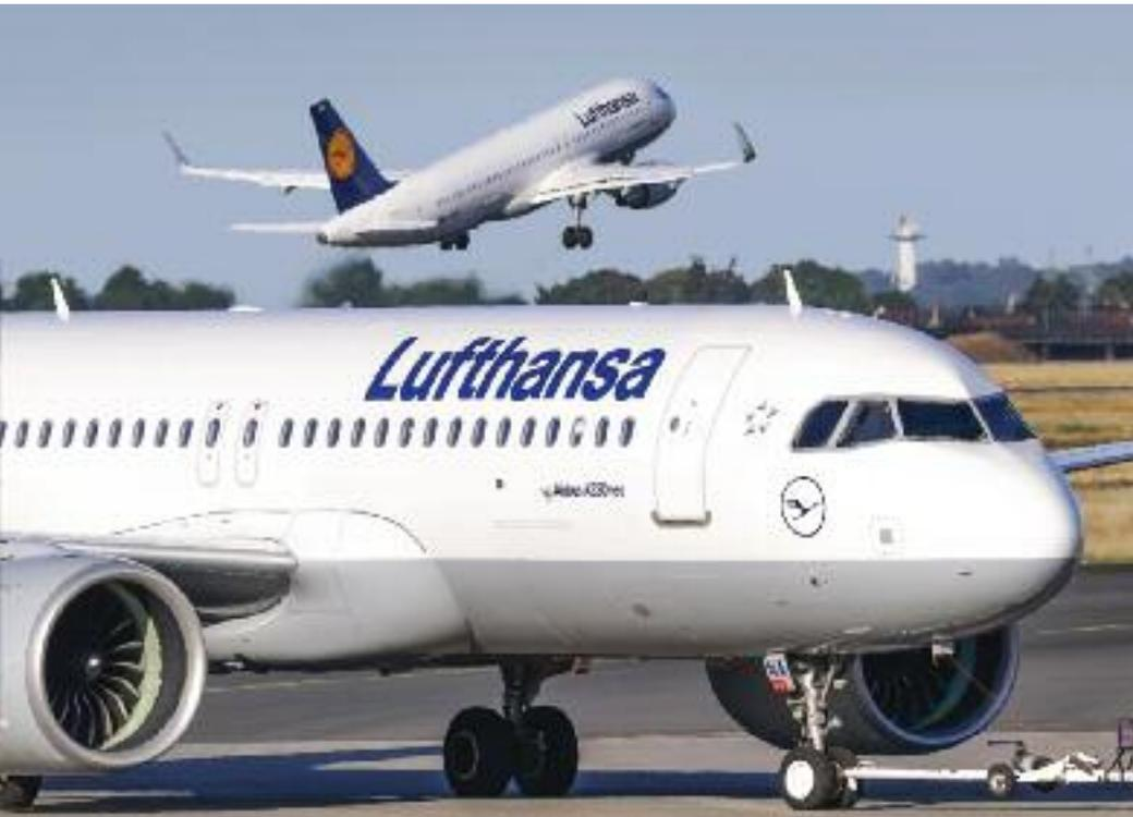
*The first A320neo entered service with Lufthansa in January 2016. Airbus claims the aircraft will provide fuel burn per seat savings of up to 20%, by 2020, compared to similar-size, previous generation aircraft.*
