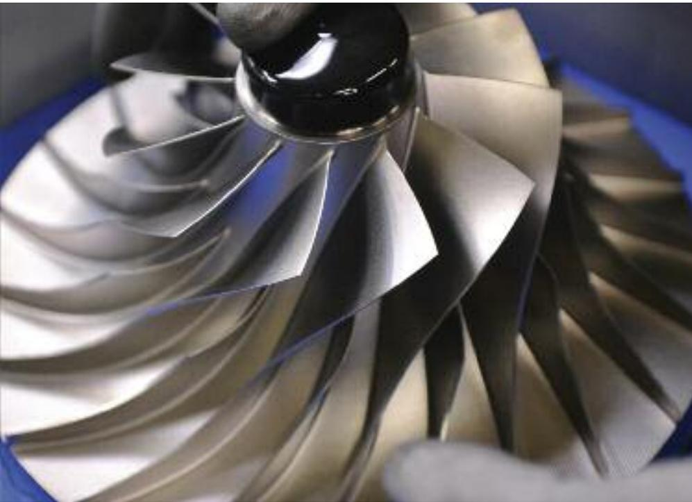
*The centrifugal compressor of a radial-configured APU is a core component. Deterioration of this and the turbine disk stages are key drivers of removal for shop visit maintenance.*
