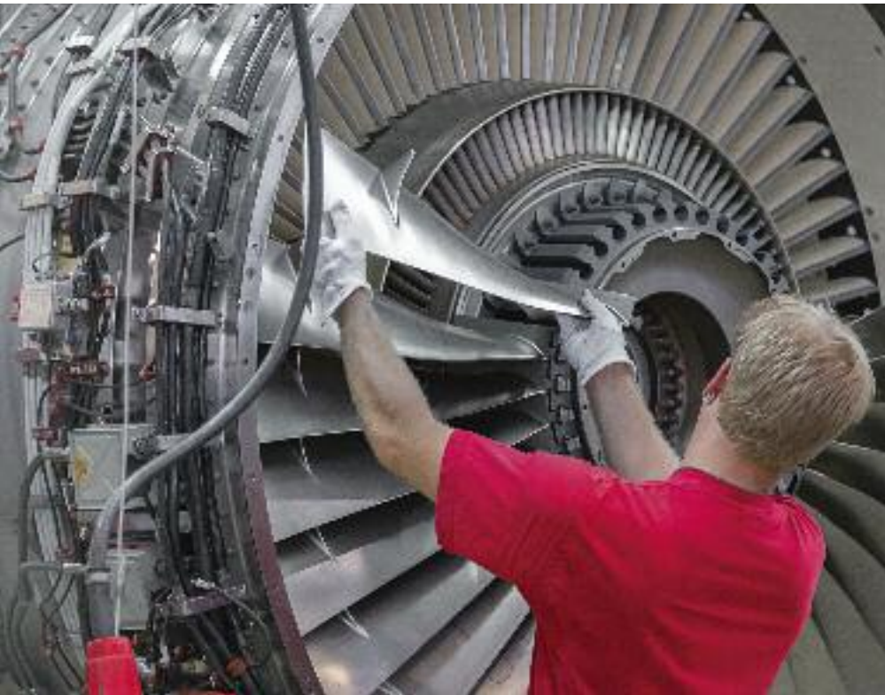
SR Technics performs maintenance and repair for the CFM56-5 and -7 series. Its Cork facility, SR Technics Airfoils Services Ltd, performs hi-tech parts repairs on LPT blades and vanes.
