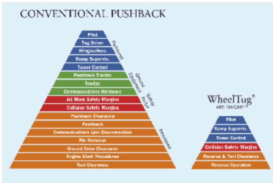
WheelTug has produced a pyramid diagram to demonstrate how the use of its system could reduce the time used for pushback. The use of WheelTug with TaxiCam removes the need for ground equipment and reduces personnel required during pushback.
