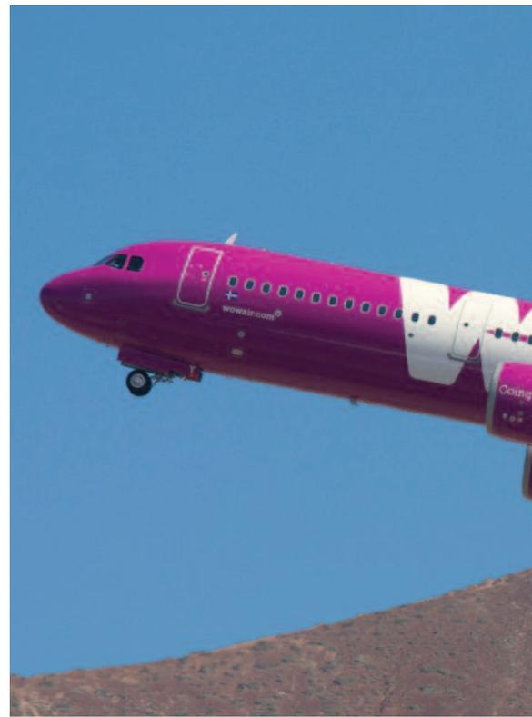
*When compared to the A321ceo, the A321neo has an absolute fuel burn that is 15-17% lower. On initial analysis, the A321neo seems to meet its initial expectations at product launch. This percentage difference between the two is enhanced in the A321neo's favour due to its higher seat count because of its ACF interior.*
