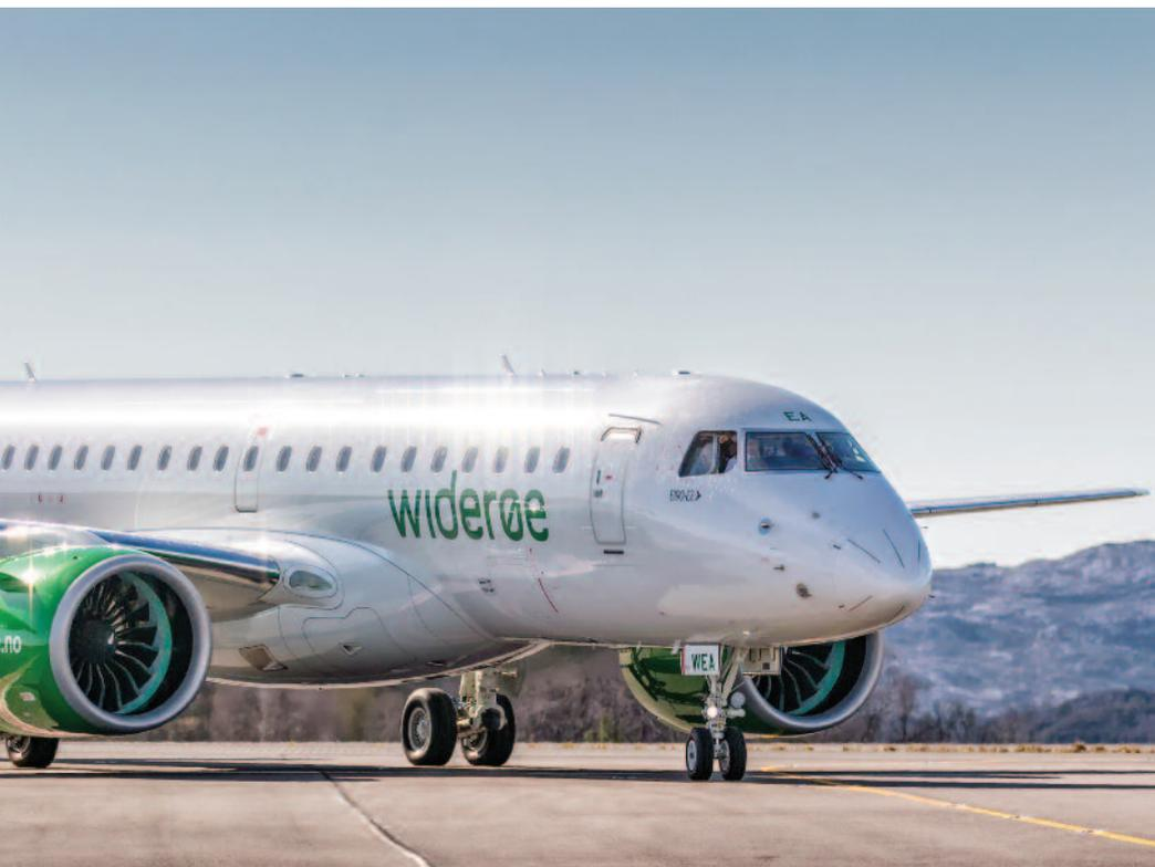
The first of the E2 jets, the E190-E2, entered into service in April 2018. The aircraft is powered by the PW1900G, which has a bypass ratio of 12.0:1. This will achieve high fuel burn efficiency, and the aircraft is expected to have a 17.3% lower fuel burn than its equal-sized predecessor the E-190 or E190-E1.
