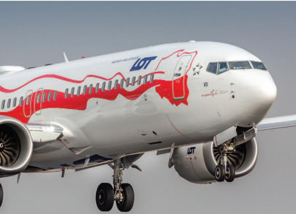
substantially heavier than the NG family, with the MAX-8 reportedly weighing in at 6,500lbs more operating empty weight (OEW) than the 737-800 it replaces. The baseline aircraft family has a range of 3,300-3,850nm depending on type, load, configuration (auxiliary fuel tanks) and flight planning rules. The range of the MAX-8 variant will be 3,500nm.
