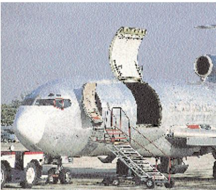
The full implications of the AD are that each pallet position will be limited to a weight of 4,000lb, the aircraft will have an altitude ceiling and cruise speed limit imposed and all containers are likely to have to be loaded so that their access doors face aft. The limitation on pallet weight may impose further payload losses because of weight and balance considerations. Pallet weight could then quite easily be less than 4,000lb.
