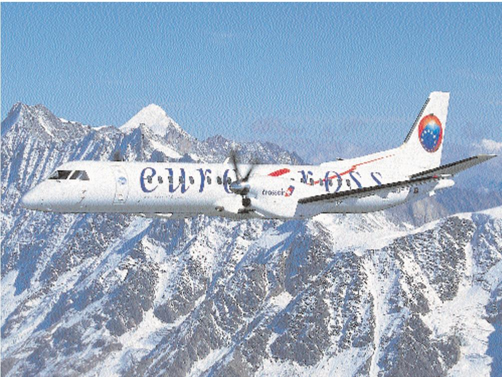
*The Saab 2000 suffered a large number of setbacks. It has longitudinal stability problems, it did not meet internal noise targets, it had a shortfall in airfield performance and experienced weight growth. These all led to late certification. The aircraft failed to penetrate the US market and won a handful of customers in Europe. This left a legacy for all would-be high-speed turboprops.*
