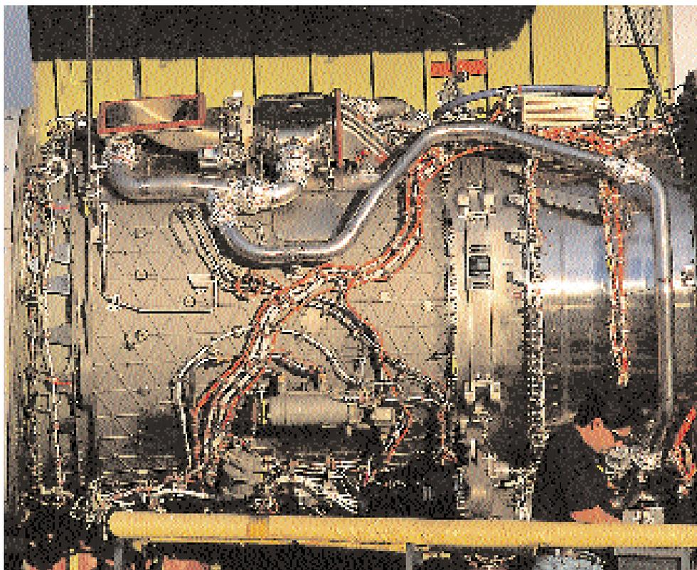
*The BR700 series is able to meet CAEP IV limits with a single-stage combustor, but there is a dual-stage combustor available for the engine.*
