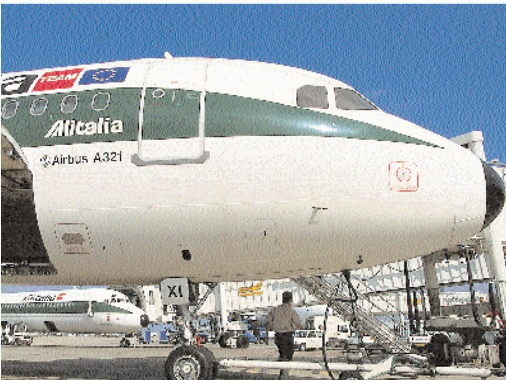
will still involve the repair and repainting of panels. The actual workscope will, however, be customer-specific. A budget of about 1,300MH for an A320 and 2,100MH for an A321 would be typical for an operator wanting to keep a clean aircraft with a pleasing appearance.
