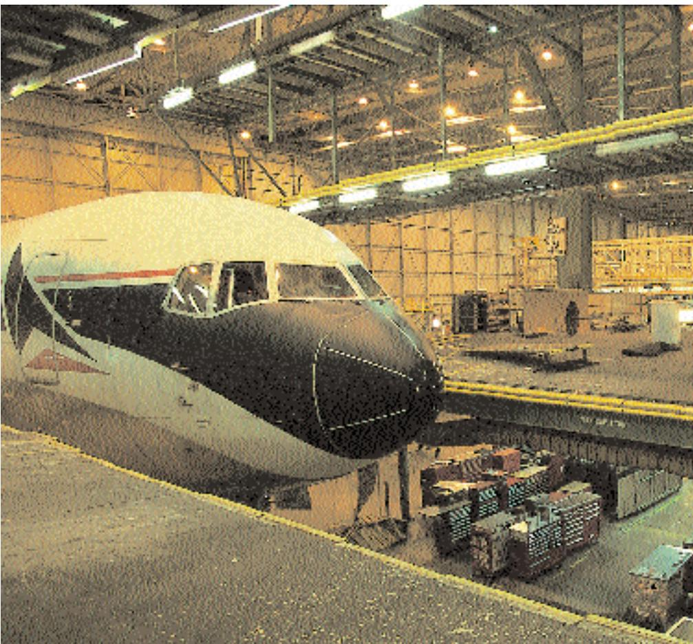
Cabin refurbishment is done every 5-6 years or fourth C check, which most operators treat as being similar to the D check. "Cabin work will include refurbishment of lavatories and galleys; repainting and recovering sidewall panels; cleaning, inspecting and recovering of seats; carpet replacement, and refurbishment of overhead bins. This usually consumes about 3,000MH.
