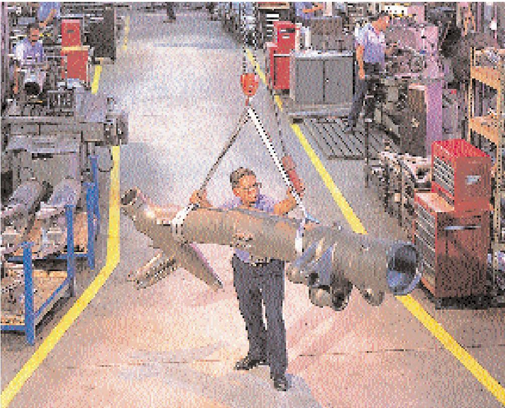
Plumbing and wiring is re-installed and the full landing gear set is tested.
