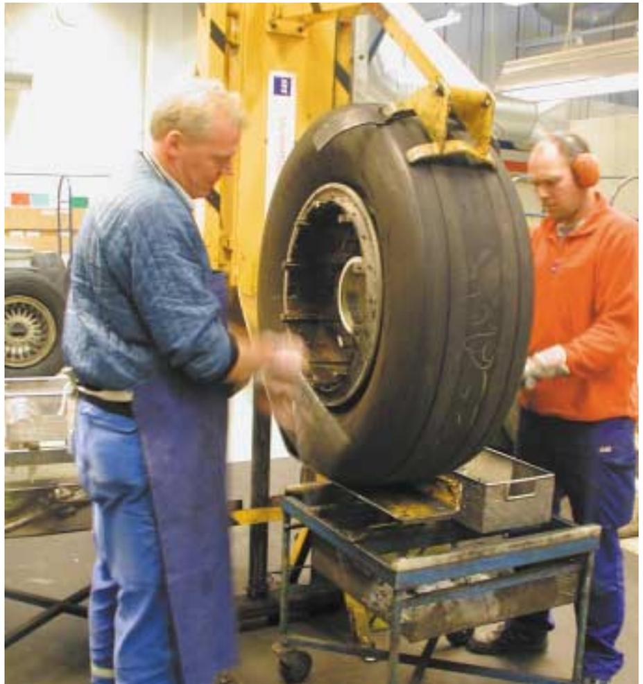
metallurgical inspection is carried out on the highest loaded areas on wheel halves,” explains Ken Hutchins, wheels & brakes marketing manager at Messier Services. “The miscellaneous hardware have a detailed inspection. This includes bolts, nuts, washers, hat shields and bearings. They are replaced if certain criteria are not met. Minor services are done every tyre removal, while major repairs are done every 1,000-1,400 cycles”.
