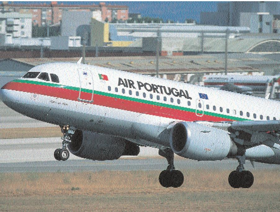
The A320 family does have its weak members, however. Initial production A320s have low MTOWs and low thrust rated CFM56-5As or V.2500-A1s. The earliest A321s are marginally Stage III compliant, and will require expensive modification to meet Stage IV.
