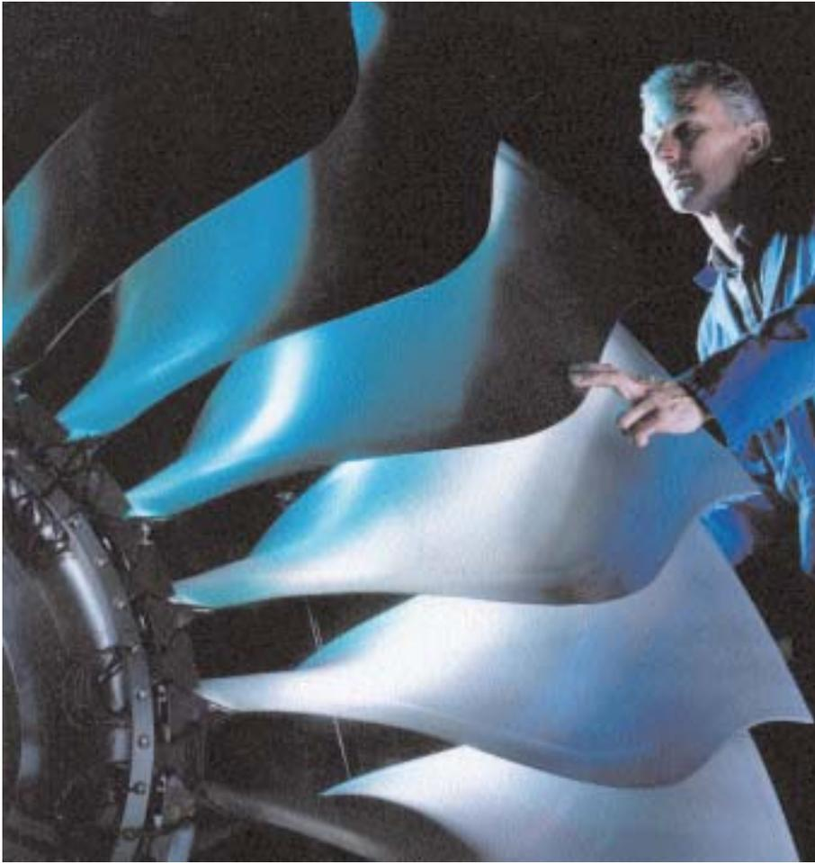
Rolls-Royce will use swept fan blades in the Trent 900 it developed for the Trent 8104. These have the effect of reducing drag, which contributes to lower fuel burn. The additional effects of swept fan blades is that less are required, reducing weight and making another contribution to reduced fuel burn.
