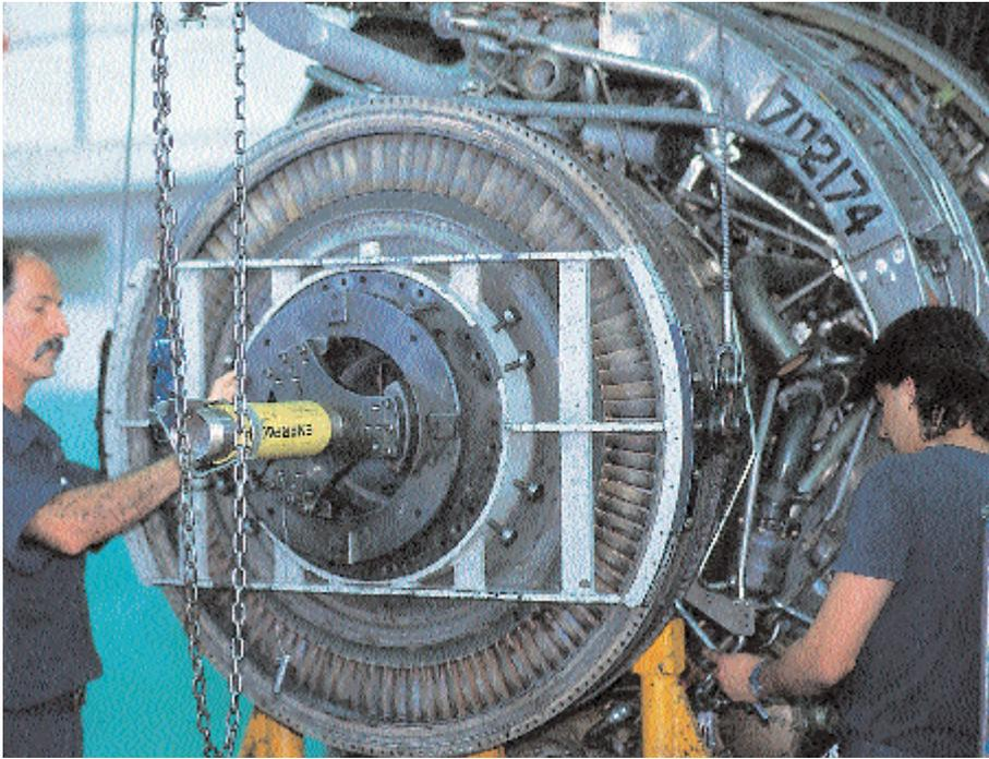
shop visit. A lighter workscope is a module level inspection and a repair as necessary. Initial inspections, however, determine if a greater workscope is required."
