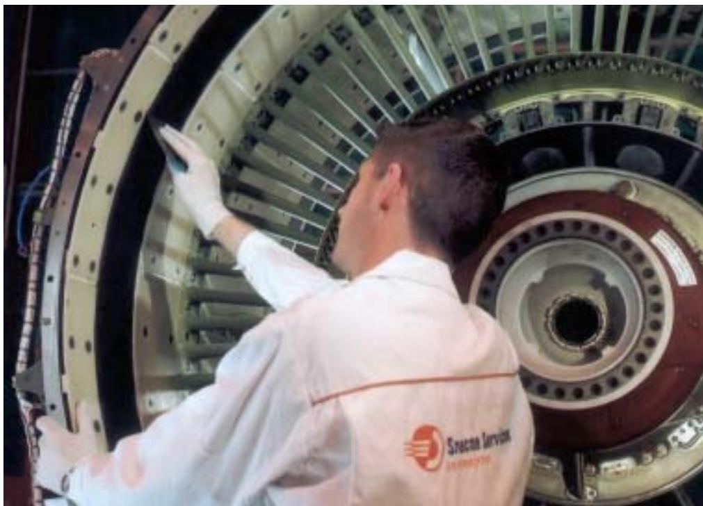
for our Salt Lake City operation, and engines come out of the shop with a margin in the region of 77 degrees. This 44 degrees margin has to be left for hot operations, and means we only get about 35 degrees of margin to use and so only get a short on-wing life of 6,000-7,000EFC. We have a disk management programme to allow for these intervals and do a core and performance restoration every shop visit, LPT every second or third visit, and fan and booster section every third visit."
