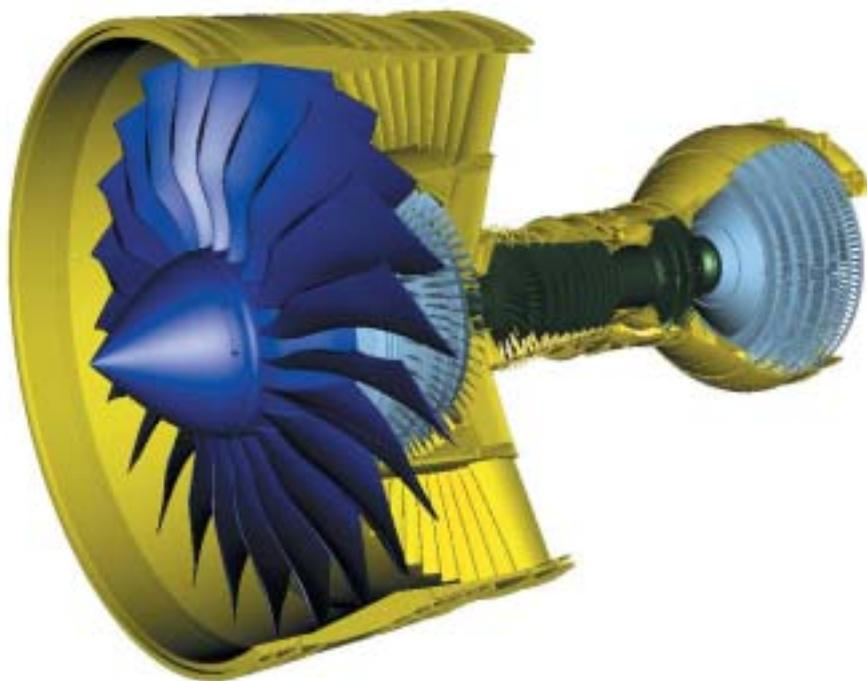
*The GENX will incorporate several new technologies. These include a third generation wide-chord composite fan, 3-D aerodynamic blades, a TAPS combustor and a contra-rotating turbine. The engine will have ratings between 55,000lbs and 70,000lbs thrust, a 112-inch diameter fan, bypass ratio of 9.5:1 and have a 15% lower specific fuel consumption compared to the CF6-80C2.*
