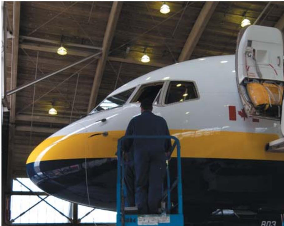
*The 757 & 767 have the same maintenance schedule. This comprises of A & C checks with system-related and structural-related tasks. Most operators combine these tasks for simplicity in maintenance planning.*
