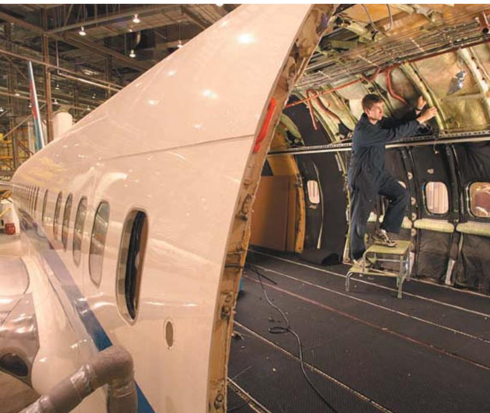
further 1,790 cubic feet of volume. This takes total available freight volume to 8,170-8,290 cubic feet. This compares to 8,390 cubic feet for aircraft converted under the Precision Conversions programme. The difference in total available freight volume between the two conversions is therefore small.
