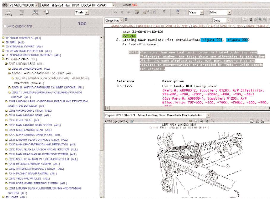
Jouve's AirGTI creates hyperlinks between OEMs' manuals that include the illustrated parts catalogue, aircraft maintenance manual and fault isolation manual.
