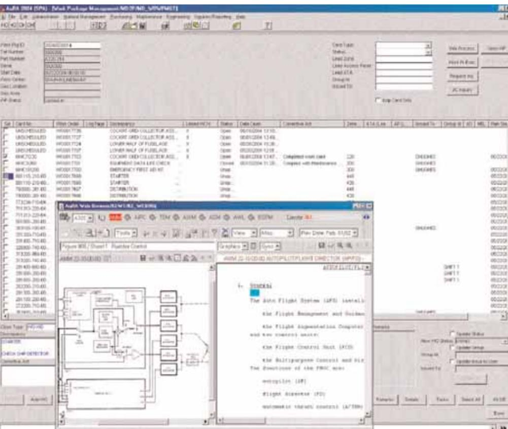
Spirent's AuRA provides mechanics with the ability to view a list of maintenance tasks, select a particular one and then access relevant pages from maintenance manuals and illustrated parts catalogues. All of this information can be accessed on a tablet computer, which has a wireless hyperlink to access the manuals.
