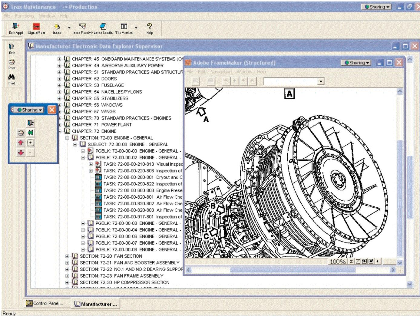
TRAX Software's system keeps the configuration of each aircraft and can store this under an ATA Chapter structure. Components and parts can then be interfaced with the appropriate pages of the aircraft maintenance manual and illustrated parts catalogue.
