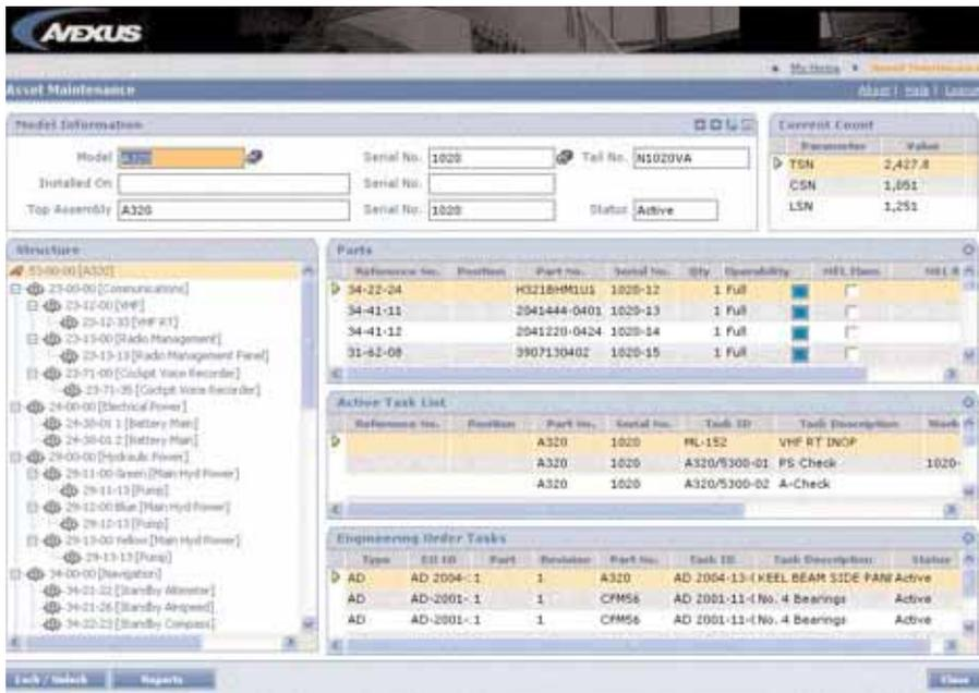
Avexus's Impresa stores an aircraft's structure down to the level of each component. The maintenance status of each component is tracked and can be viewed, as can the maintenance task cards.
