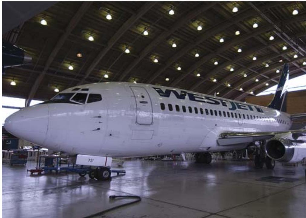
Transit checks are performed before the first flight of each day, and pre-flight checks before all other flights in the day. Daily checks are usually done overnight every 24 hours. Assuming an annual utilisation of 2,600FH and 2,500FC per year, the aircraft will operate an average of seven flights per day. Excluding grounded time for maintenance, the aircraft will have about 350 daily checks, 350 transit checks and 2,150 pre-flight checks each year.
