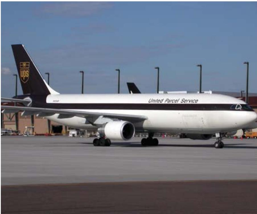
*The CF6-80C2 is rated between 52,500lbs and 61,500lbs of thrust and operated in a wide variety of roles. These can be short-haul operations where average cycle times are 1FH, and well as medium- and long-haul operations with average cycle times as high as 8.0-10.0FH. Engines operated on short-haul missions have on-wing times in the region of 2,500-3,500FC.*
