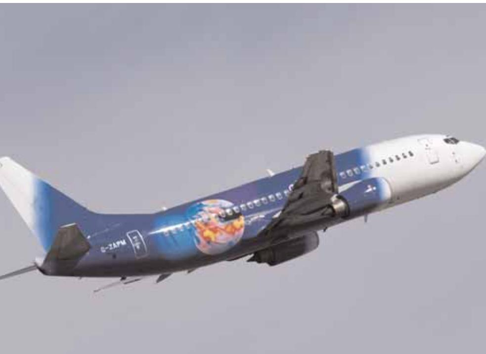
*The majority of 737s are -300s. Half of these are powered by the CFM56-3B1, while just less than 300 are equipped with the -3C1 engine. Many -300s have now reached mature age.*
