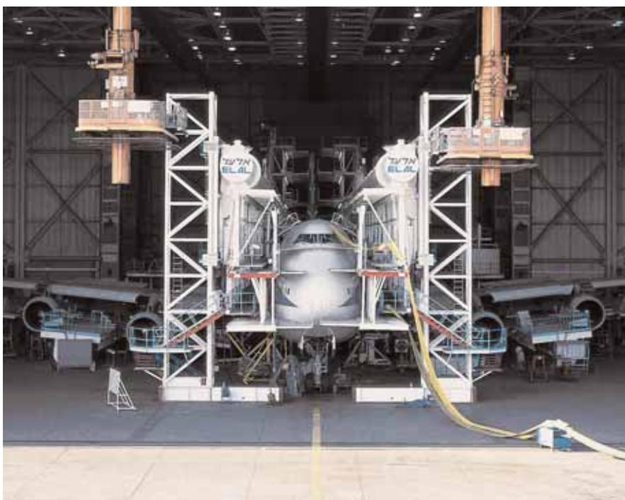
*The 747-200's/-300's ageing aircraft programme adds a large number of MH to base checks. Full workpackages for D checks can be 90,000-100,000MH for aircraft at their D4 or D5 checks.*
