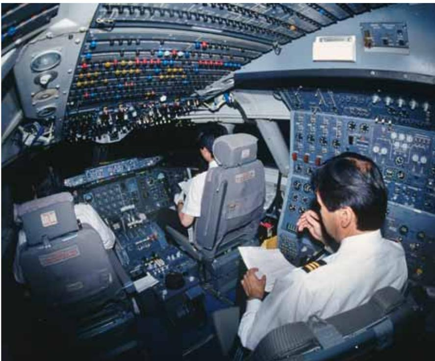
*ECM data was traditionally recorded manually by flightcrews, and only during take-off and once in the cruise. ECM data is recorded automatically on modern aircraft. It can even be recorded and transmitted to ground stations in real-time.*
