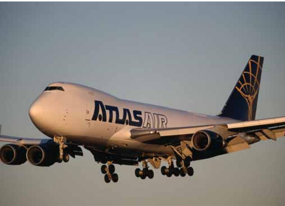
*Converted 747-400s will have virtually the same main deck space for accommodating pallets and containers as -400Fs. The 747-400SF will only have a side cargo door, and not a nose door. There are two conversion programmes and three engine types, resulting in six different structural payloads varying between 247,000lbs and 250,500lbs.*
