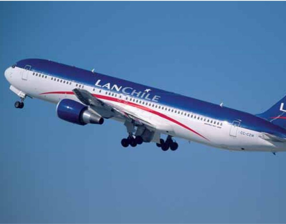
80C2B2/B4/B6/B7. These engines were rated between 52,500lbs and 60,800lbs to power aircraft with gross weights between 360,000lbs and 412,000lbs.
