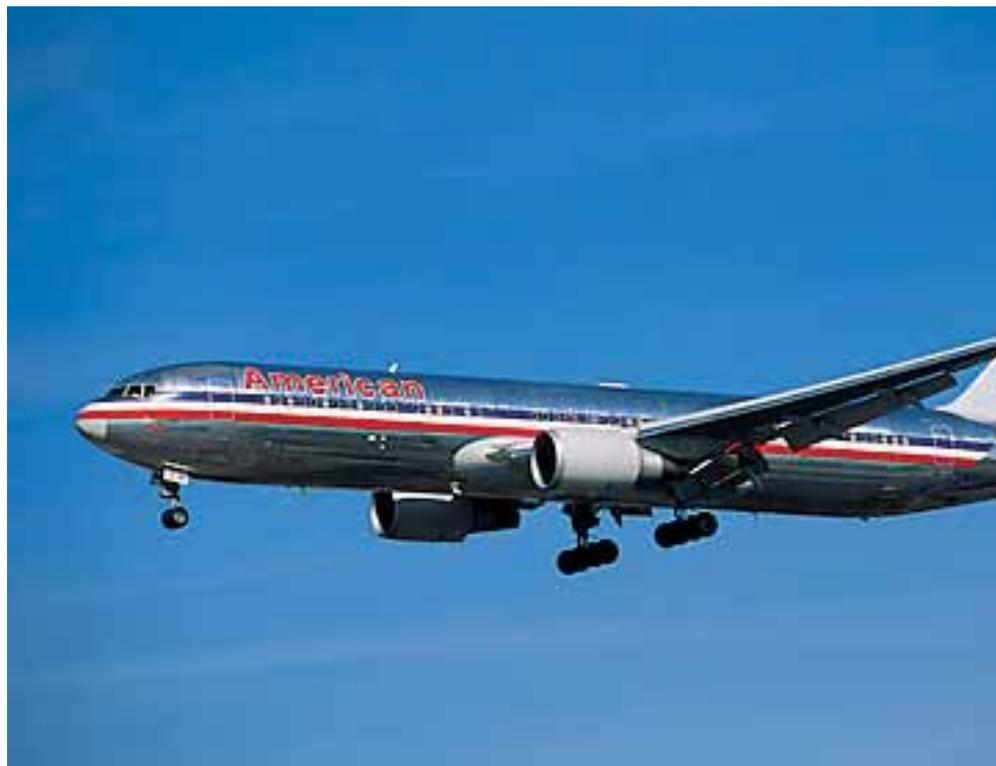
*The -300ER is the most numerous of all 767 models, accounting for 501 out of 745 passenger-configured aircraft in service. The majority of these have CF6-80C2 engines.*
