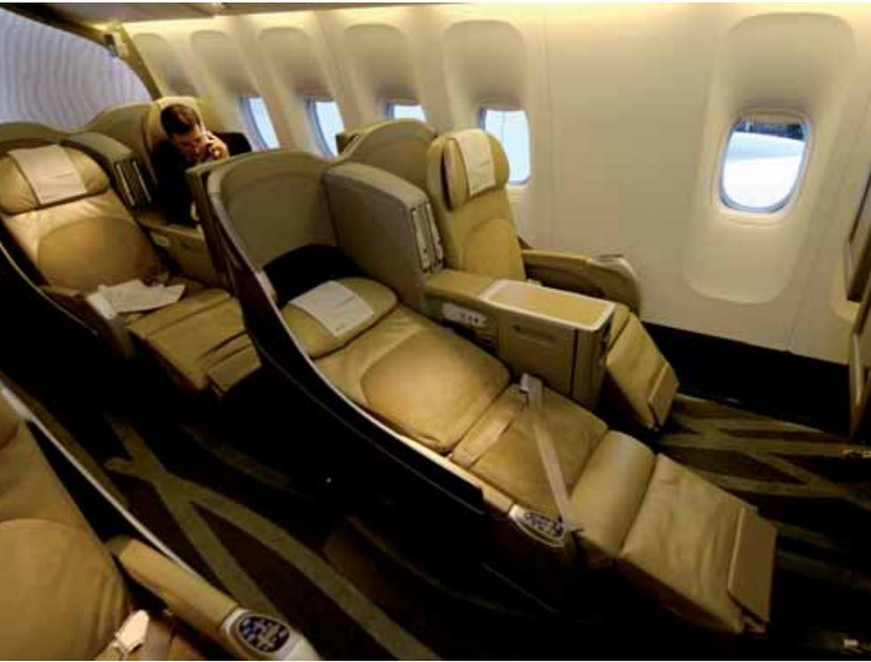
*Lower grade lie-flat seats are positioned at an incline, with the end of the bed passing underneath the seat in front. This type of seat, however, allows overall seat numbers to be maintained or increased.*
