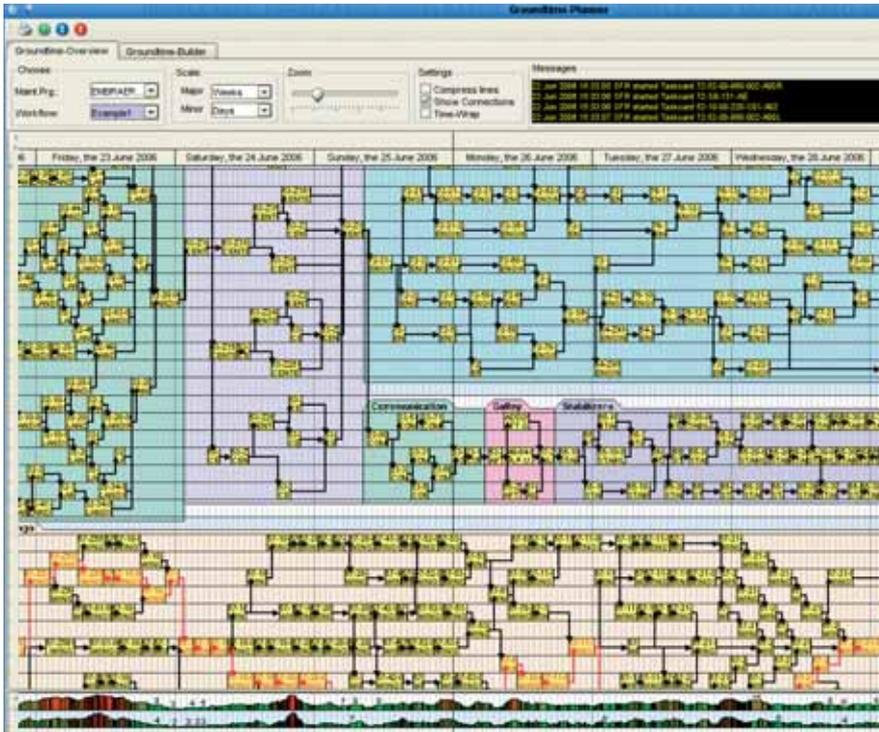
The AMOS integrated MRO software system includes a graphical task planning tool. This helps production planning staff to monitor and resequence jobs as a hangar check progresses, always keeping in mind the critical path that determines whether the aircraft is completed on time.
