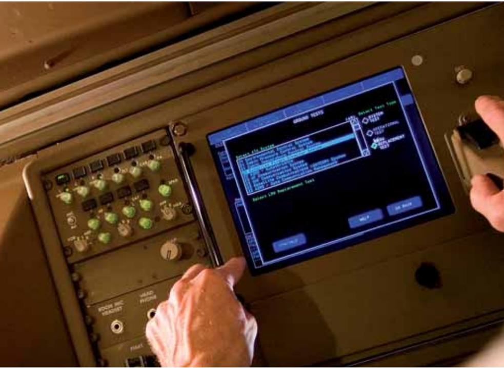
EICAS. “The CMC can display these results on the MCDU, or downlink them to ground stations via ACARS,” says Borges. “The CMC also provides an integrated user interface to perform ground tests on all connected systems. The experience used from this system on the 747-400 led to the development of the next generation of on-board maintenance computer.”
